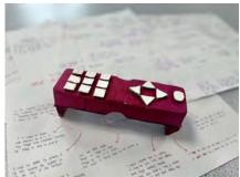
Using the practical skills developed through previous projects students were tasked with realising their designs to create a high-quality prototype out of foam and card that would allow for high quality testing and future development.
